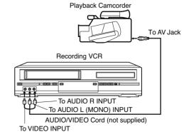
For duplicating a previously recorded tape from a camcorder, follow the camcorder manufacturer's instructions. A typical camcorder dubbing hookup is shown above.
